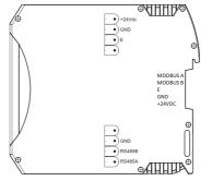
+24VDC **GND** RS485A Modbus, 250 nodes **RS485B** MODBUS A Modbus, 32 nodes **MODBUS B E** passing-through item
