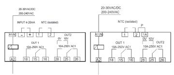
The neutral must always be connected to terminal A1.
